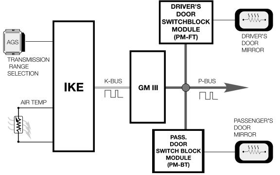
The reverse gear tilt feature for the passenger's mirror is signaled from the GM III, over the P-bus, when reverse is selected and the mirror switch is set for the driver's side.
